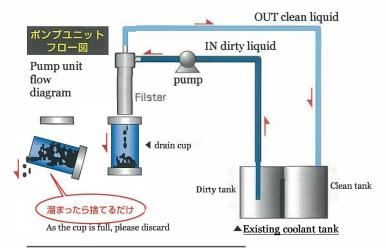
The dirty liquid intake, 10 micron level filtration, clean liquid discharge, capturing sludge, all these functions will work after only turning on power. All automated unit, **ALL-IN-ONE!**
