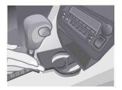
Used in the automotive cup holder's push/pull function. The object can be operated with constant force.
