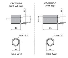
Note) When attaching, make sure that the side without a bearing chamfer is the impact surface.
