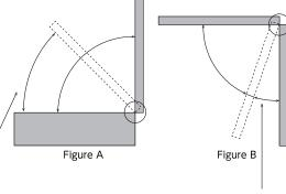
Stronger damper torque allows the lid to close gently until it is fully closed.
