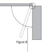
Stronger damper torque prevents the lid from being fully closed.
