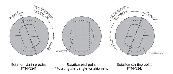
6. There are dampers that generate torque in either the clockwise or counterclockwise direction when the rotating shaft is seen from the above. Select a model according to use.
