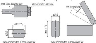
⟨Recommended dimensions for mounting the rotating shaft⟩
