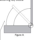
Stronger damper torque allows the lid to close gently until it is fully closed.
